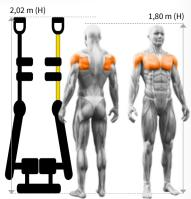
The Rear Delt / Pec Fly is equipped with adjustable, rotating arms, which should adapt to the arm length of different exercisers and offer the right training posture. The independent adjustment crank on both sides not only offer different starting positions, but also provide more variety in training. The long and narrow back padding provides support for the back during the Pec Fly and for the chest muscles during the training of the delta muscles.
